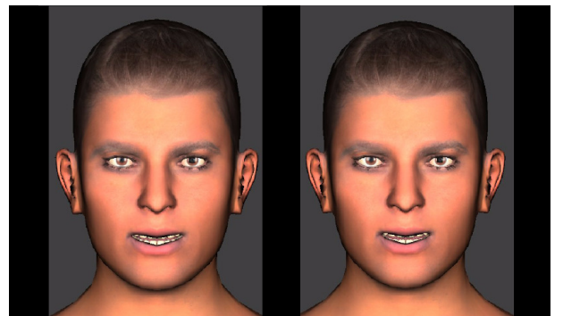
Figure 7: Example frame taken from a video used in the perceptual test. In this case the left and right avatars were driven by k -means and minimum deviation decision trees, respectively. The frames show the articulation of the sound "K".
